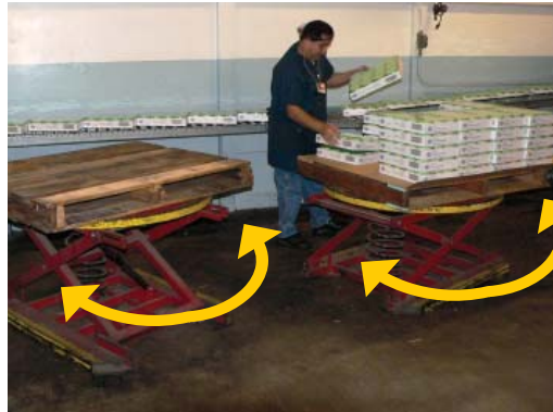
Turntable on a load leveler
